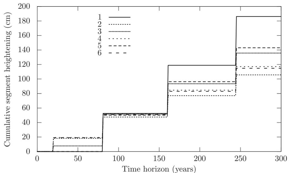
Figure 1 Cumulative segment heightenings for a dike ring with six segments.
