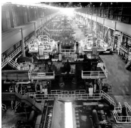
Figure 1 The hot strip mill with glowing hot slab of steel.
